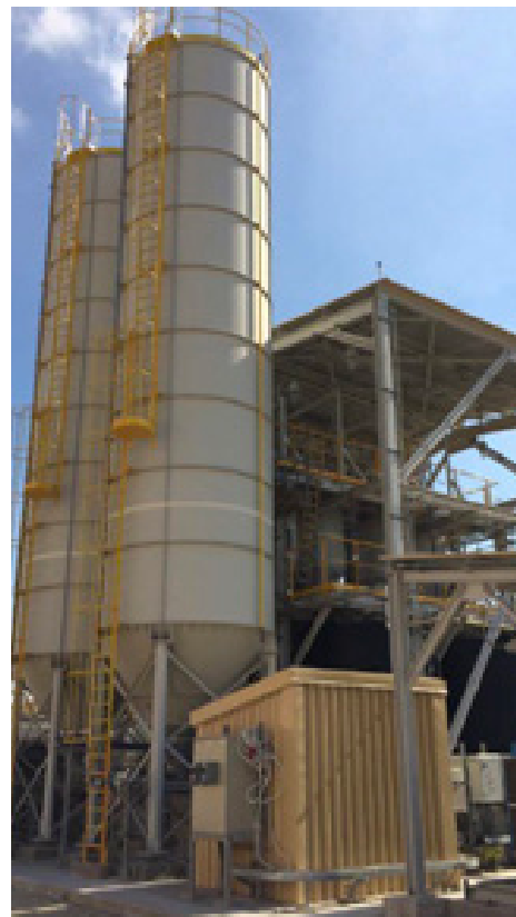
OPTIFLEX 6200 C used for level measurement of hydrated lime powder in vertical cylinder silos.
