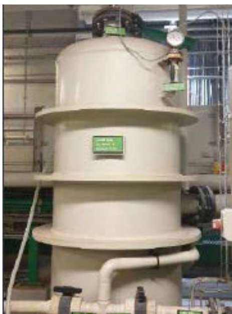
OPTIFLEX 7200F used for measuring sugar condensate.
